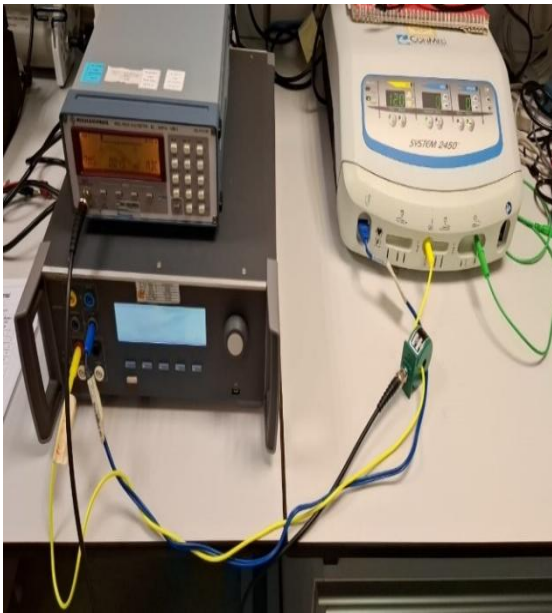
Figure 12: Monopolar Cut current and Power Measurement Connection
