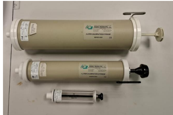
Figure 8: Calibrated Syringes for Lung Capacity Calibration
