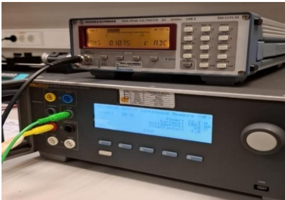
Figure 19: Bipolar coagulation test end cable connection.
