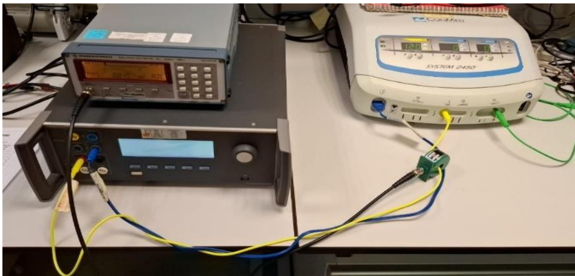
Figure 16: Monopolar Coagulation test end cable connection.
