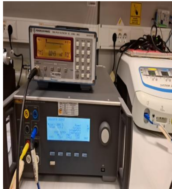
Figure 13: Monopolar Cut current and Power Measurement Connection
