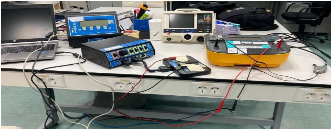
Figure 29: Calibration set of Standard Reference and UUT Defibrillators with charge pads and load module and a laptop.
